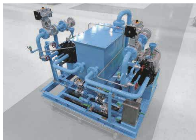
Condenser Vacuum Pump 40VDP45.5, 5.5 kW × 1800 min -1 (S.S) 2.42 m 3 /min × 40 kPa (abs)
