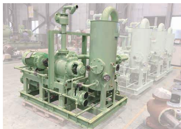
Condenser Vacuum Pump 80V-F615, 15 kW × 1150 min -1 2.78 m 3 /min × 64 mbar (abs)
