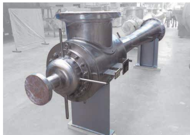
Steam Ejector for Condenser Gas Extraction System
