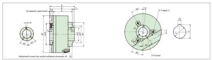
Note: For TGM20 and below models, the angle of 45° marked with an asterisk (\*) is 60°. For TGM6 and below models, there are two P screws on the mounting seat side, one at the keyway portion and one to the left of it.
