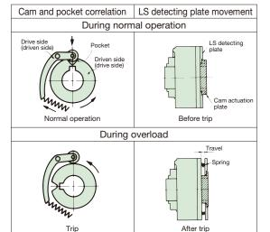
Torque is transmitted by the two-point-contact engagement of the cam follower and pocket
