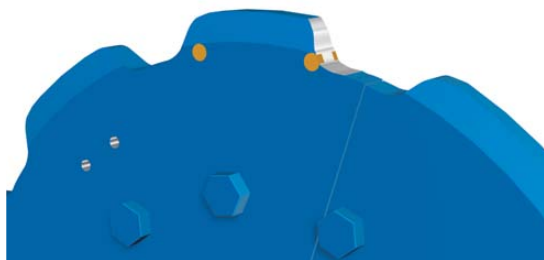
Tooth profile wear and indicator pins
